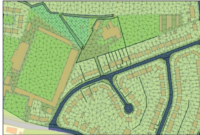
Figure 6. Image illustrates the porous walls added to the model to increase the accuracy of representation of the fences and walls. The blue areas represent the mesh zones that were used to lower the roads thereby representing the kerbs.
